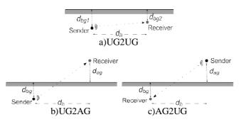
•Underground to underground (UG2UG) Link: Both the sender and the receiver are underground buried and communicate via soil. This type of communication is used for multi-hop information delivery and is the main focus of this work.
